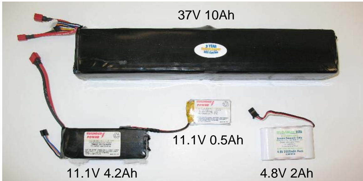
Figure 9: USL Testbed Batteries
