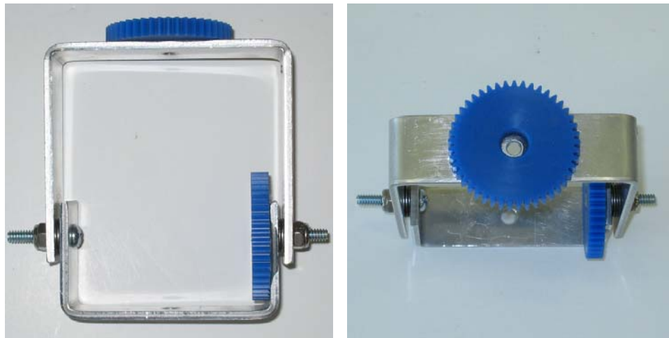
Figure 26: Assembled Pan/Tilt Camera Brackets with Gears
