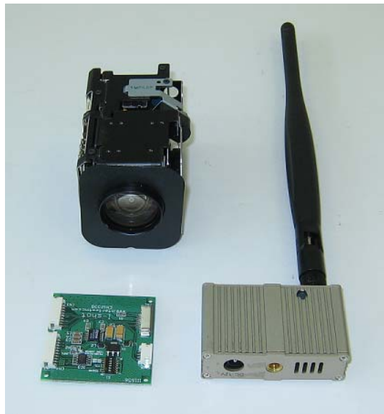
Figure 12: Sony FCB-EX980S Camera, Interface Board, and Video Transmitter
