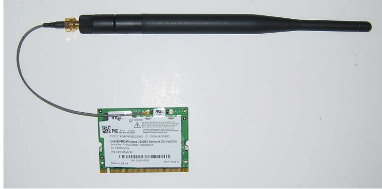
Figure 11: Intel Pro 2200 with External Antenna and Pigtail
